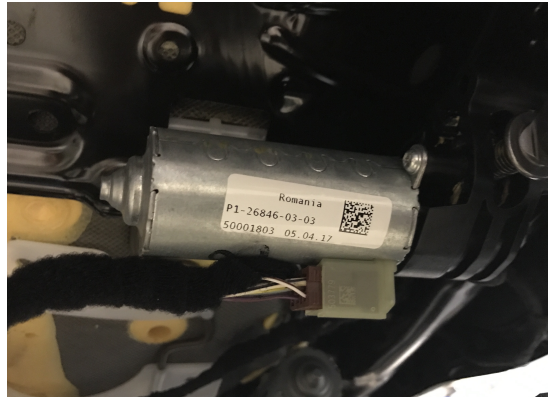
Figure 4.2: Image of a Nidec 12V 405.940 (P1-26599-01-03) motor
