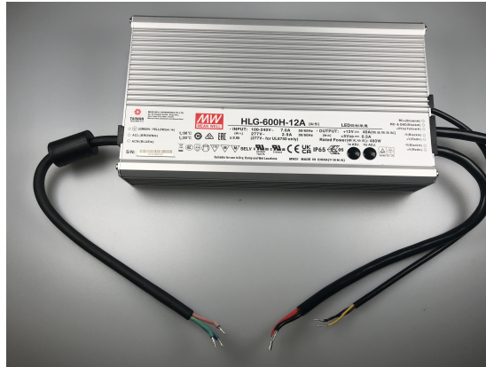
Figure 4.5: Image of a Mean Well HLG-600H-12A power supply
